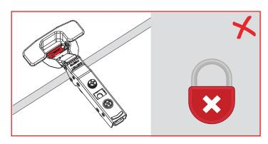
Locking mechanism should not be rotated in the base of the hinge cup during insatllation of tool-less hinges.
