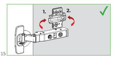
Hinges should be mounted to the door first, then attached to the mounting plate on the cabinet.
