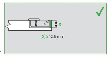
Cup depth should be min. 12,5 mm.
