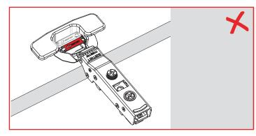
Tool-less hinges should not be closed with extreme force during installation.
