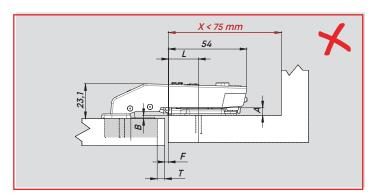
In the assembly of 90 degrees hinges, the distance in the cabinet should not be a shorter than 75 mm.
