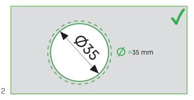
Cup diameter should be drilled 35 mm exactly
