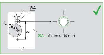
Tolerance size of dowel hole should be max. +0.1 mm
