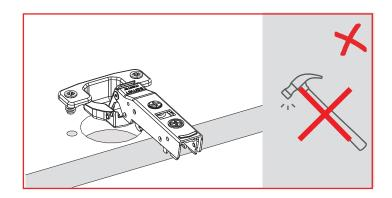
Metal hammer should not be used during assembly of hinges with dowels
