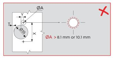
Tolerance size of dowel hole should not be larger than +0.1 mm.
