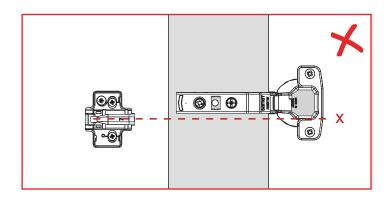
Hinge and mounting plate should not be on different axis
