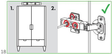
Cabinet should be levelled before adjustmet
