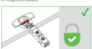
Tool-less mechanism should be open during installation of tool-less hinges.
