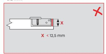
Cup depth should not be lower than 12,5 mm.
