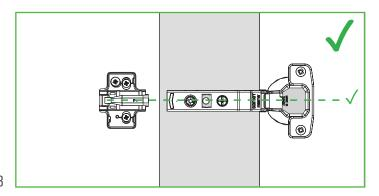
Hinge and mounting plate should be on same axis
