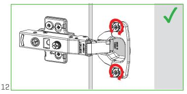
Easy Fit installation screws should be in the un-locked position prior to installation.
