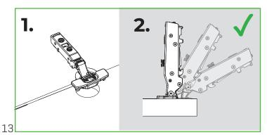
Tool-less hinges should be closed gently to install hinges to the door.
