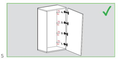
Assembly should be started from bottom side for high cabinet doors
