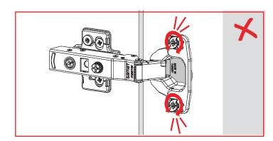
Easy Fit installation screws should not be rotated past the locked position during installation.
