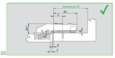
In the assembly of 90 degrees hinges, there should be a minimum 75 mm distance in the cabinet
