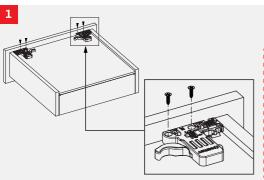
**Note:** Use angled holes to mount SMART LOCK when wooden floor width is selected less then 12 mm.
