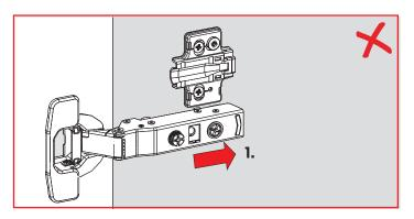
Hinges should not be mounted to the mounting plate on the cabinet first.
