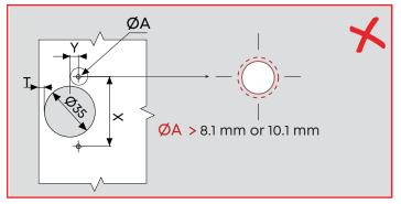
Tolerance size of dowel hole should not be larger than +0.1 mm.
