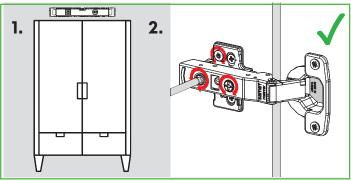
Cabinet should be levelled before adjustmet
