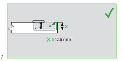
Cup depth should be min. 12,5 mm.
