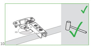
Plastic hammer should be used during assembly of hinges with dowels
