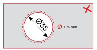
Cup diameter should not be drilled larger or smaller than 35 mm.
