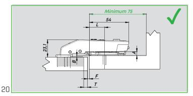
In the assembly of 90 degrees hinges, there should be a minimum 75 mm distance in the cabinet
