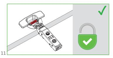
Tool-less mechanism should be open during installation of tool-less hinges.
