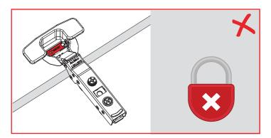
Locking mechanism should not be rotated in the base of the hinge cup during insatllation of tool-less hinges.
