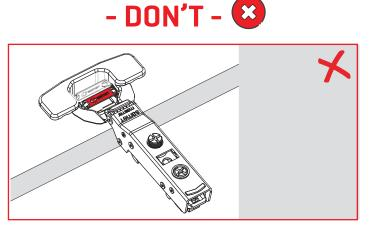
Tool-less hinges should not be closed with extreme force during installation.
