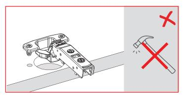
Metal hammer should not be used during assembly of hinges with dowels
