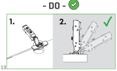
Tool-less hinges should be closed gently to install hinges to the door.
