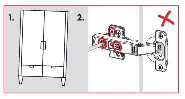
Cabinet should not be levelled after adjustmet
