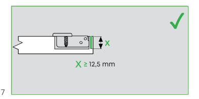
Cup depth should be min. 12,5 mm.
