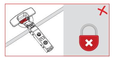
Locking mechanism should not be rotated in the base of the hinge cup during insatllation of tool-less hinges.
