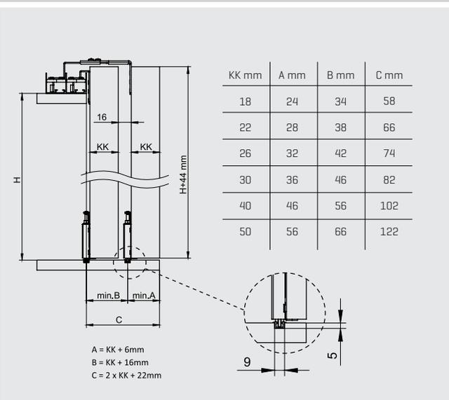
Bottom Rail Assembly and Fixing
