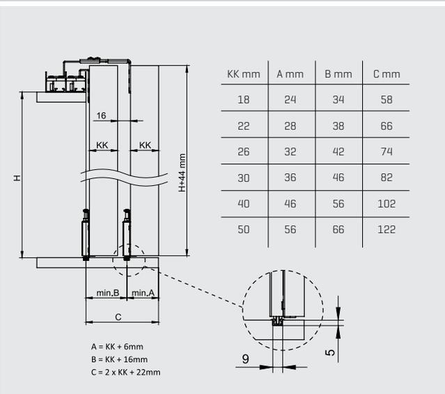
Bottom Rail Assembly and Fixing
