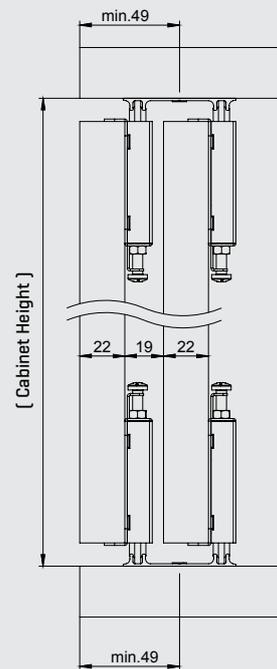
NOTE: DIMENSIONS SHOWN IN BRACKETS ARE VALID FOR "18 mm" AND "22 mm" DOOR THICKNESSES.
