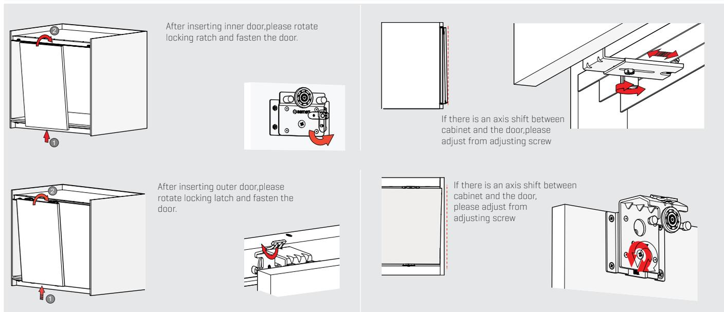
After inserting inner door, please rotate locking ratch and fasten the door.
