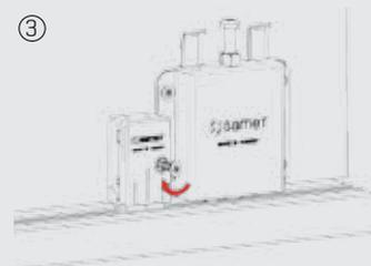
\* Doors should be balanced before the assembly of stopper.
