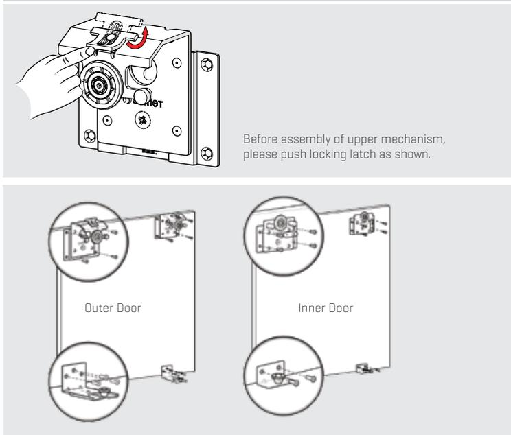
Before assembly of upper mechanism, please push locking latch as shown.
