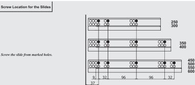
Screw the slide from marked holes.
