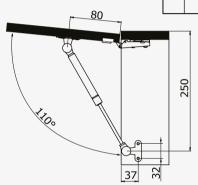
Mounting measurement for rounded conncecting element.
