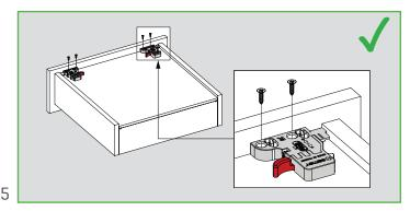
Locking mechanisms should be installed flush up against the drawer sides.
