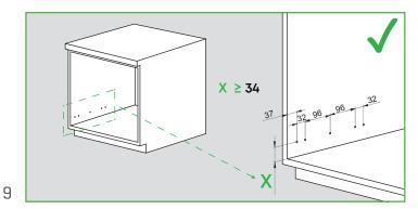
The lower drawer should be installed a minimum of 34 mm (1-20/32") up from the cabinet bottom panel for soft close version.
