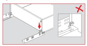
Back hook of the slide should not be bent as it is inserted into the drawer back.
