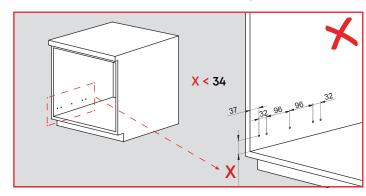
The lower drawer should not be installed lower than 34 mm (1-20/32") up from the cabinet bottom panel for soft close version.
