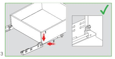
Back hook of the slide should be inserted into the drawer back gently.
