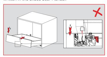
Plastic safety pin should not be in the locked position before the drawer is set in place. The safety pin should not stay in the unlocked position after the drawer is set in place.
