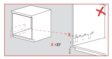
Slides should not be installed further than 37 mm away from the front edge of cabinet for overlay applications.
