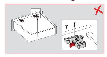
There should not be any gap between the locking mechanisms and the drawer sides.
