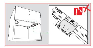
Welded sheet metal should not be bent on Slidea push-open mechanisms.
