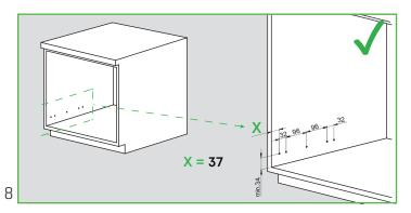
Slides should be installed 37 mm back from the front edge of the cabinet for overlay applications.
