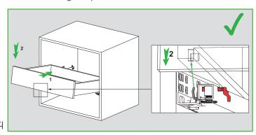
After inserting the back hook of the slide gently, the vertical metal pin should be fitted into the vertical hole after the drawer is laying flat on the top of the slides.
