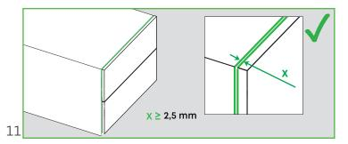
Drawer front gap should be a minimum of 2.5 mm on Slidea push-open models to ensure proper functionality.
