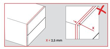
Drawer front gap should not be less than 2.5 mm on Slidea push-open drawer models to ensure proper functionality.
