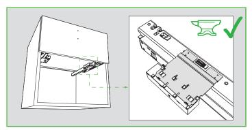
Pay close attention to welded sheet metal on Smart Slide Full Power push-open mechanisms.
