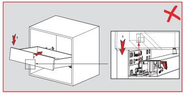
Do not insert the drawer before the back hook on the slides has been inserted, and be careful to avoid bending the vertical metal pin.
