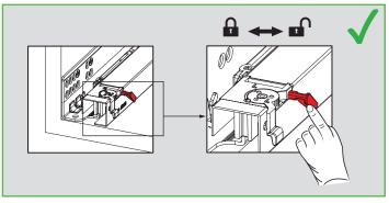
Plastic safety pin should be switched to the unlocked position before the drawer is set in place. Then the safety pin can be locked into the horizontal hole on drawer side panel.
