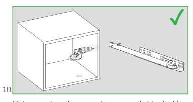
Make sure there is no sawdust or wood chips inside the slides.
