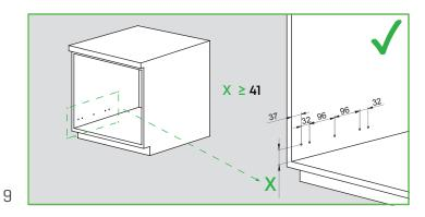
The lower drawer should be installed a minimum of 41 mm (1-20/32") up from cabinet bottom panel for the soft close version.
