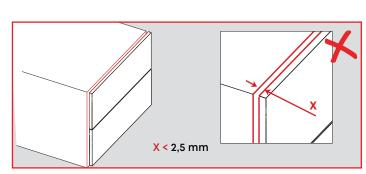
Drawer front gap should not be less than 2.5 mm on Smart Slide Full Power push-open drawer models to ensure proper functionality.
