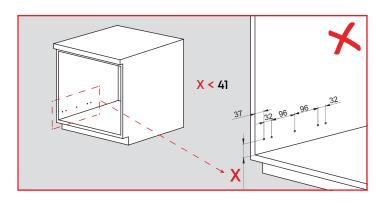
The lower drawer should not be installed lower than 41 mm (1-20/32") up from cabinet bottom panel for the soft close version.
