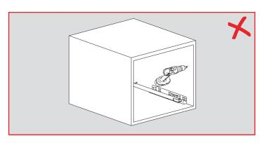
There should not be any sawdust or wood chips inside the slides.
