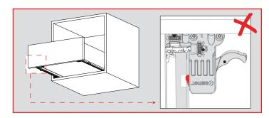
The drawer should not be fixed to the 1st stage of the locking notch.
