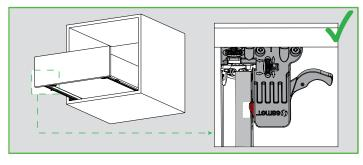
The drawer should be fully inserted to the 2nd locking notch.
