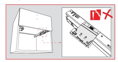
Welded sheet metal should not be bent on Smart Slide Full Power push-open mechanisms.
