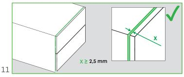
Drawer front gap should be a minimum of 2.5 mm on Smart Slide Full Power push-open models to ensure proper functionality.
