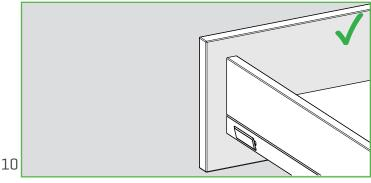
Attach the outer decorative covers by inserting the placement guides gently into place from the top down.
