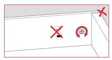
Power drill or power screwdrivers should not be used on adjustment screws.
