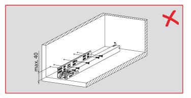
Slides should not be installed 40 mm up from cabinet bottom panel.
