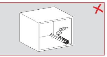
There should not be any sawdust or wood chips inside the slides.
