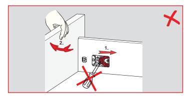
Screwdrivers should not be used to remove the drawer front.
