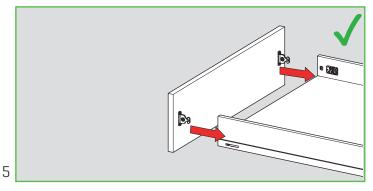
Before installing the drawer box, the drawer front should be attached to the drawer sides.
