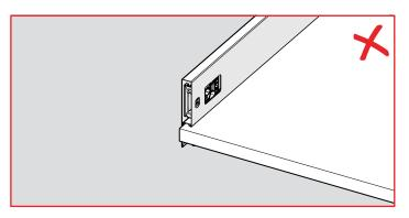
The front edge of the drawer bottom panel should not protrude past the front of drawer sides.
