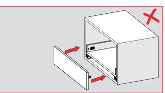
Drawer fronts should not be attached after the installing the drawer box.
