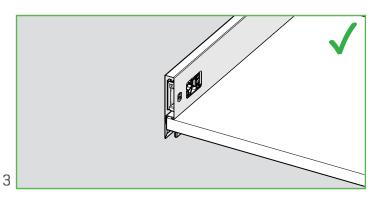
The front edge of the drawer bottom panel should be flush with the front side of drawer sides.
