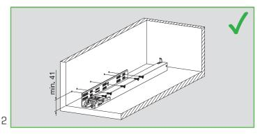
Slides should be installed a min. of 41 mm (1-20/32") up from cabinet bottom panel.
