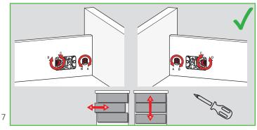
Adjustments should be made carefully by turning the adjustment screws in opposite directions to achieve your desired adjustment.
