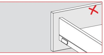
Upper placement guides on the outer decorative covers should not be installed from the bottom up.
