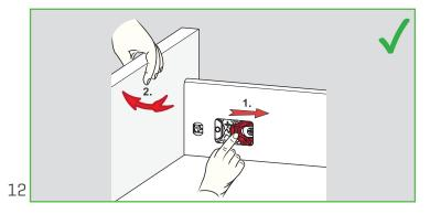
To remove the drawer front be sue to pull back the removal switch completely until it stops.
