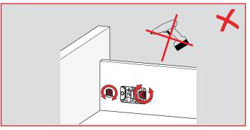
Adjustments should not be made with a power drill or power screwdriver.
