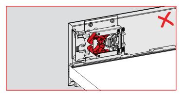
Verify that the lock mechanism is not in the closed position before attaching the drawer front.
