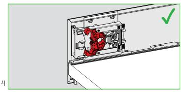
Verify that the lock mechanism is in the open position before attaching the drawer front.
